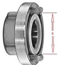
To determine the correct size of a STORZ coupling face a measurement between the two lugs on the coupling face as shown (left) must be taken.
